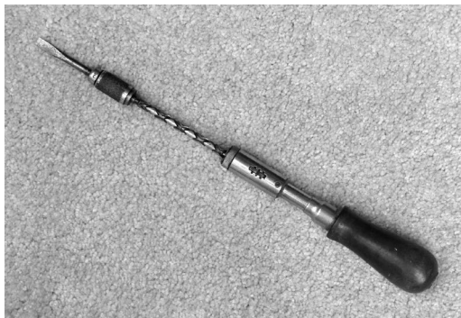
Fig. 12-1. A “Yankee” screwdriver. The chuck holding the screwdriver blade is constrained to rotate clockwise as the handle is pressed inward with one hand while the other hand holds the knurled, freely rotating sleeve next to the chuck. The helical grooves on the shaft are crisscrossed so that sliding the tab on the steel body toward the handle constrains the bit to turn counterclockwise, thereby loosening a screw. The middle position of the tab prevents internal rotation.
